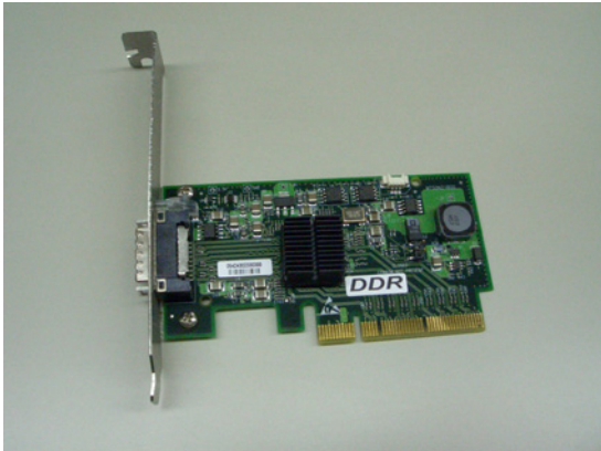
図1 Mellanox Technologies 社の PCI Express 対応 DDR InfiniHost HCA MHGS18-XT DDR Fig. 1 InfiniHCA HCA MHGS18-XT DDR for PCI Express bus from Mellanox Technologies, Inc.
