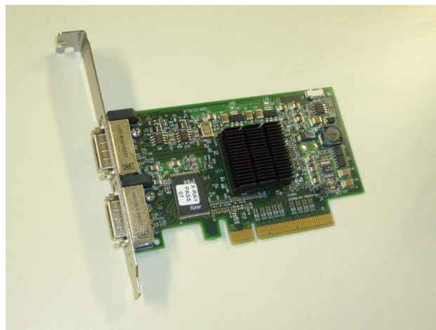
Figure 4: InfiniHCA HCA MHEA28-XT for PCI Express bus from Mellanox Technologies, Inc.
