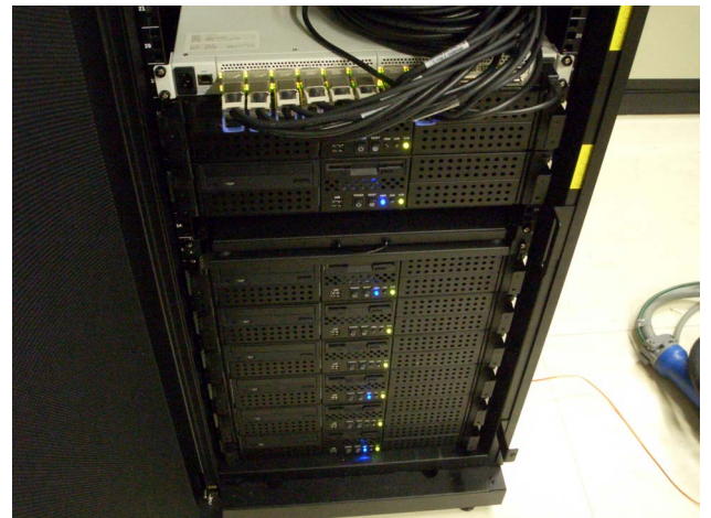
Figure 6: HDAM Express based Opteron Cluster IBD connected with InfiniHost HCAs and MTS2400.
